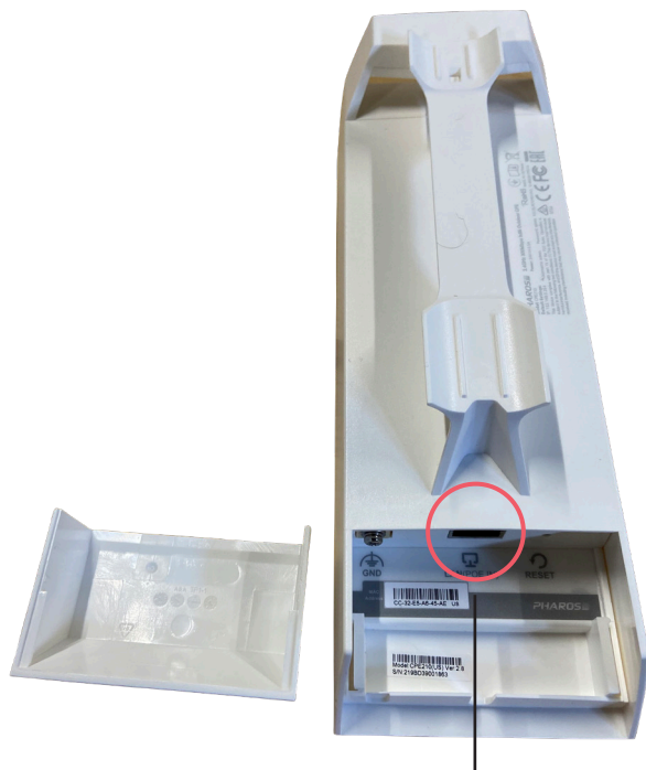
Ethernet connection from PoE
